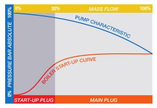
However, when the boiler is starting from cold the requirements from the valve are totally different. As the valve is required to control a small mass flow with a high delta P, the required rangeability can no longer be realised by one valve alone. Potential cavitation will easily damage the valve.
