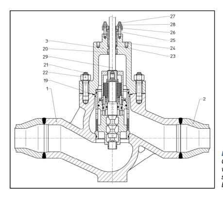
Left: Combi feed water control valve, 4 stage start up trim, single stage main control, BWE.
